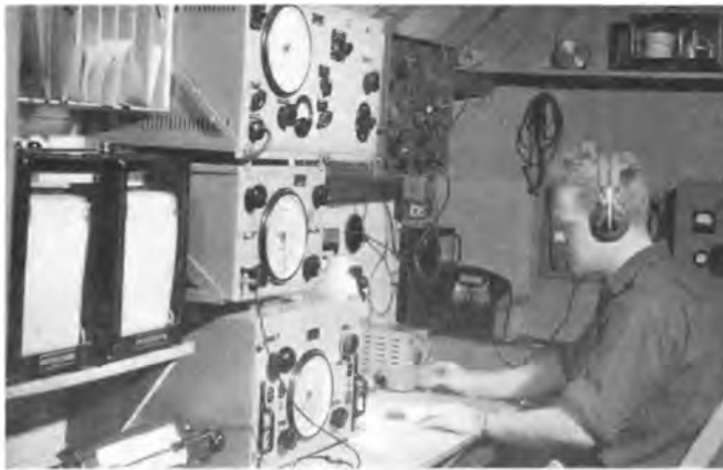
Borge Haagensen operates a small radio station at Nord in 1952: Danish Transmitter and 2 Danish Receivers. Behind these, a BC-654 Transmitter.
