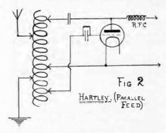
where it was located on 50 metres! As soon as the choke coil was inserted the wave-length returned to normal, and no further difficulty was experienced. The grid choke was made by winding 20 turns of ordinary bell wire on a pencil.
